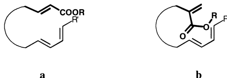
Figure 1. Two types of dienophile substructures in IMDA reactions: (a) crotonate type dienophile; (b) methacrylate type dienophile
